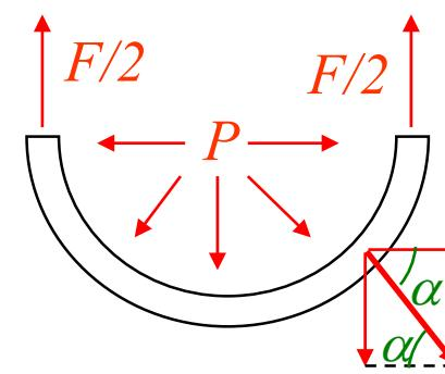
A diagram of a vessel end showing internal pressure  $P$ .
