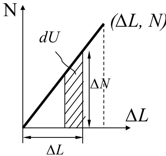
$$\left. \begin{aligned} U &= \int_0^L dU = \int_0^L N \cdot d(\Delta L) \\ Hooke \quad N &= S \cdot E \cdot \frac{\Delta L}{L} \end{aligned} \right\} U = \frac{E \cdot S}{L} \int_0^L \Delta L \cdot d(\Delta L) = \frac{E \cdot S}{2L} \Delta L^2 \Rightarrow U = \frac{1}{2} N \cdot \Delta L$$
